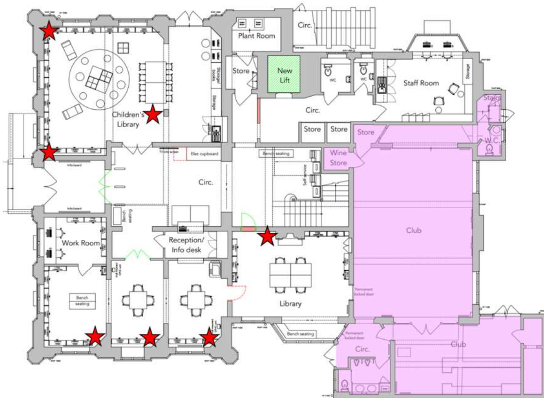
Figure 4: Ground Floor Option 4 Layout – Proposed Displacement Ventilation Outlet Locations
